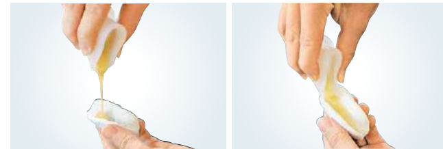
Due to high liquidity, the resin can be poured in to the fine details of the Silicone Core.
